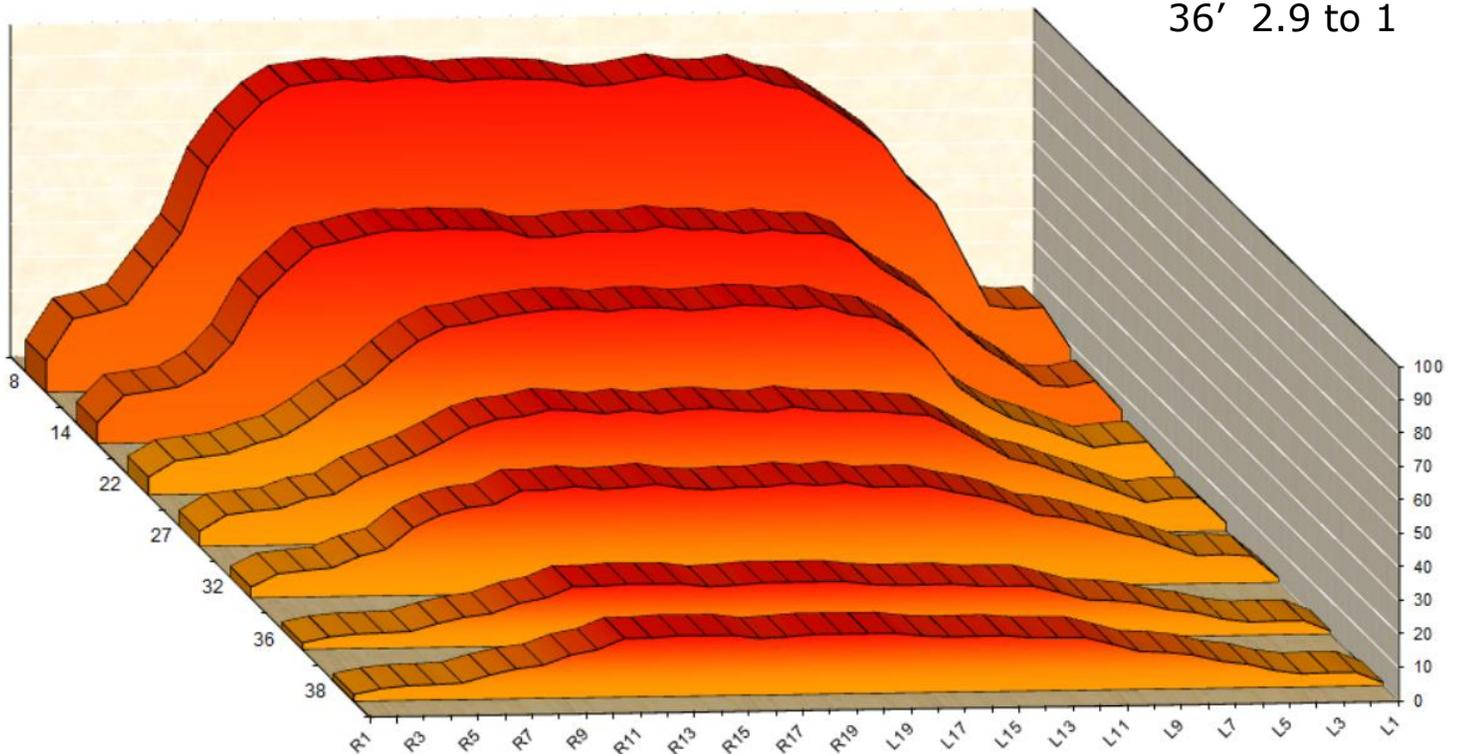
The 2D Chart above was generated by the Lane Reader showing select tapes and ratios at key distances throughout the oil pattern. USBC Sport Bowling ratios are calculated at 22' and 2' before the end of the oil pattern. **KEGEL KODE Ratios** are determined by the highest Sport Bowling ratio number for that oil pattern.
